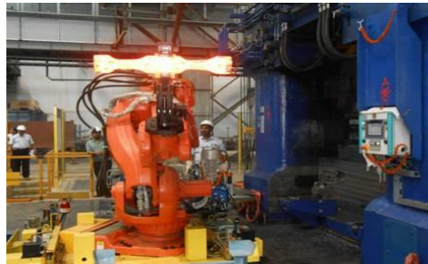
12500 Ton – SMS Meer, Germany, Wedge Press
